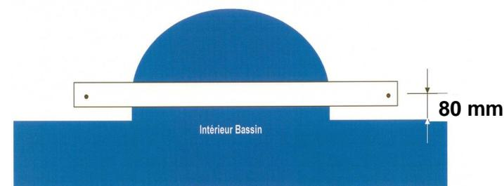
**AVERTISSEMENT** : LA CONFORMITE DU PRODUIT PAR RAPPORT A LA NORME DEPEND DU RESPECT DE LA TENSION DU DISPOSITIF D'ANCRAGE ET DONC DU RESPECT DES COTES DE PERCAGE INDIQUEES SUR LE SCHEMA CI-DESSUS.
